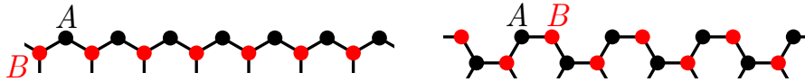
Figure 2.3.: Special types of graphene boundaries: Zigzag (left) and armchair (right). Sublattices A and B are represented by black and red dots, respectively.
